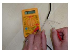
**Please Note:** If any of the readings are not within the correct tolerances the cable should be replaced. Please call the Technical Department for further details – tel: +44 (0)1530 813396
